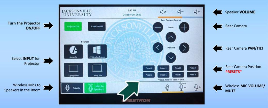
\*To set <u>Rear Camera Position Presets</u>, hold Preset Button for <u>3 seconds</u>. Repeat for Presets 2-8 for different camera angles at the touch of a button.
